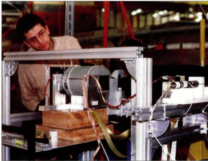
Beam testing at CERN for a carbon-fibre transition radiator used in conjunction with silicon strip detectors and a permanent magnet to separate the particles from the emitted X-ray transition radiation.
