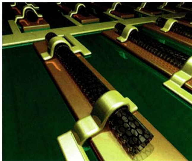
Nanologic – a carbon nanotube field-effect transistor.
